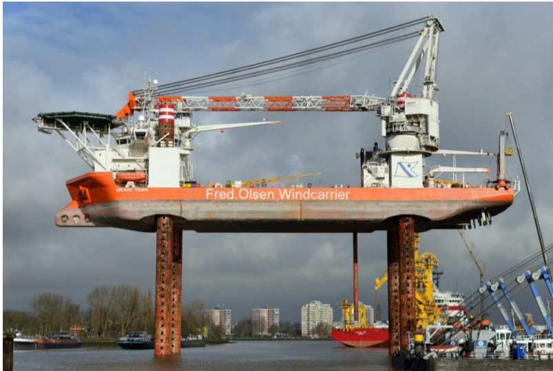
Fred. Olsen Windcarrier's Brave Tern vessel will rise above the waters near Block Island to assemble the wind farm. Image credit: Fred. Olsen Windcarrier
