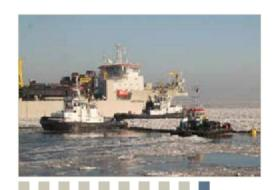
This new mega trailing suction hopper dredger has a hopper capacity of 46,000 m³. Together with its sister vessel 'Leiv Eiriksson', these hoppers are the largest hoppers available on the world dredging market. This vessel can work in water depths of up to 155 m, a new record in deep dredging.
