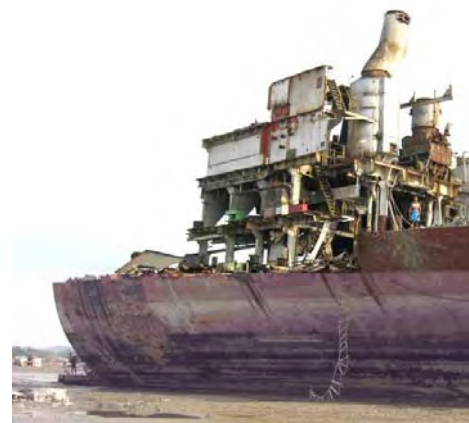
Risky extraction of an engine and shaky access to the upper level © Robin des Bois – October 2010
