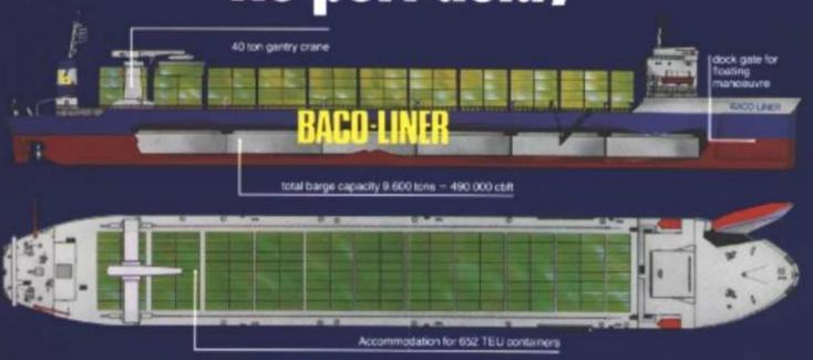
This type of vessel was specially designed for West African ports. BACO-Liner operations are unaffected by port congestion and no waiting time is involved in the smooth efficiency of this unique transport system.
